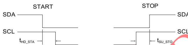
Figure 2: I 2 C STOP and START Conditions; START: A High "1" to Low "0" Transition on the SDA Line While SCL is High "1" STOP: A Low "0" to High "1" Transition on the SDA Line While SCL is High "1".
